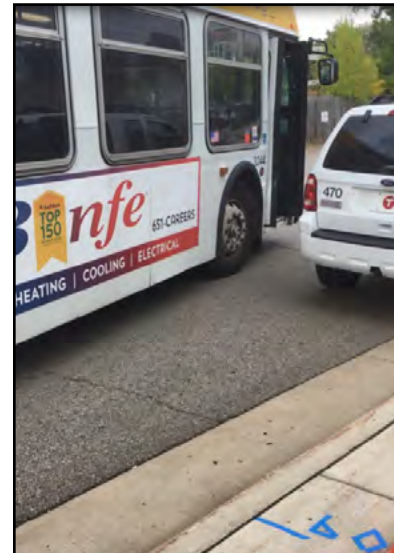
Figure 70 Screenshot showing a 60' bus testing a 10' merge zone (too short) for a far side stop and failing
