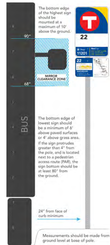
Figure 25 Bus stop sign and bus stop pole installation
