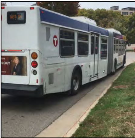
Figure 69 Screenshot showing a 60' bus testing a 20' merge zone (too short) for a near side stop and failing
