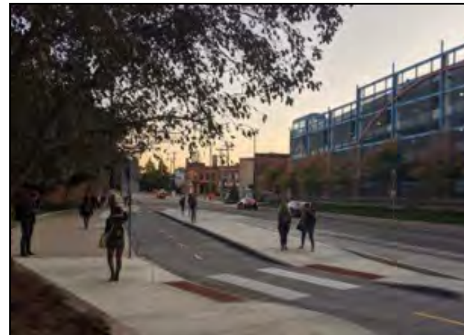
Figure 50 A floating bus stop on the University of Minnesota Twin Cities campus
