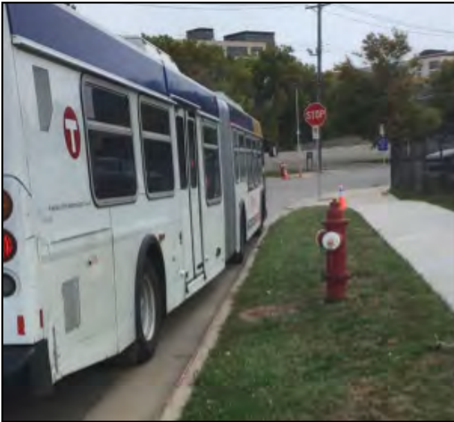
Figure 68 Screenshots showing a 60' bus testing a 40' merge zone a near side stop and a 60' bus testing a 40' merge zone at a far side stop
