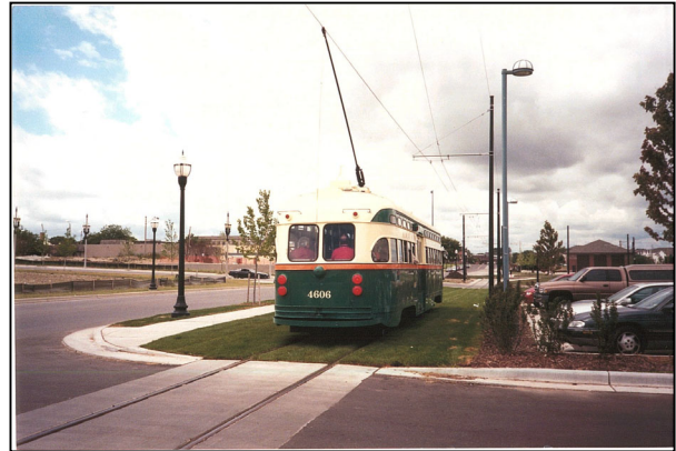
Kenosha Wisconsin Line showing unobtrusive nature of overhead wires. Wires could be attached to decorative poles.
