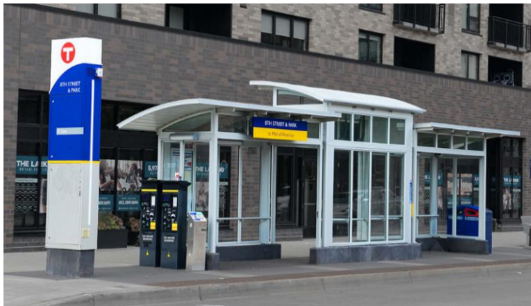
Large shelter 36 feet long, 5 feet wide, and 9-12 feet high
