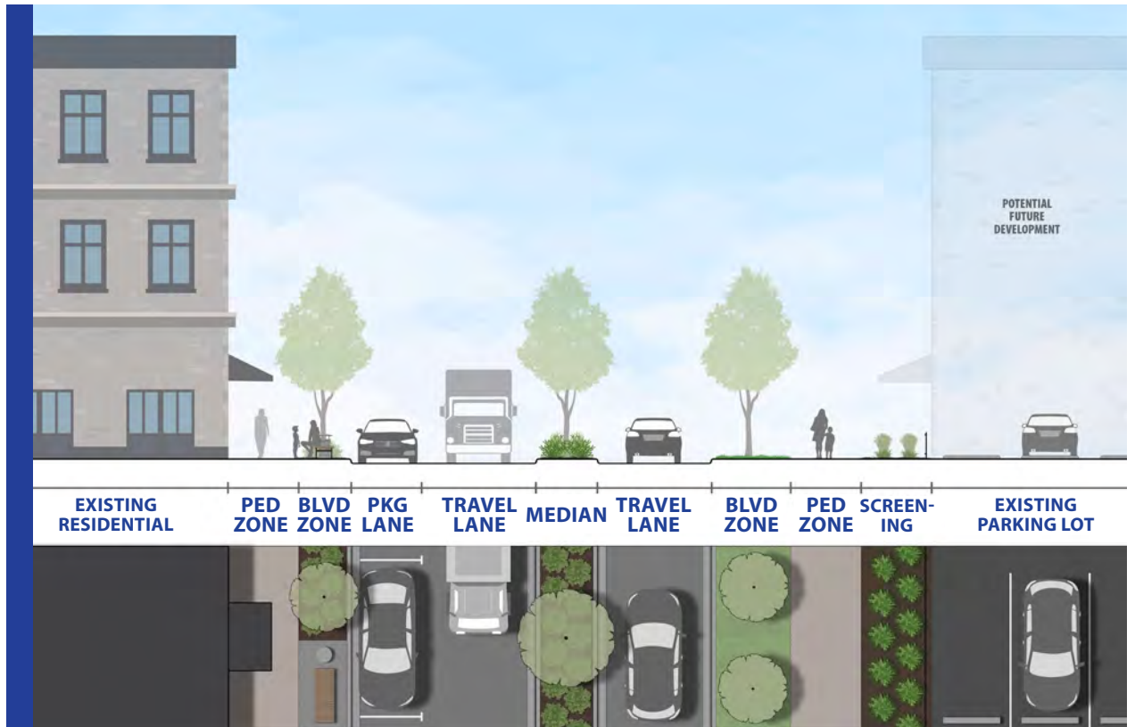
Figure 3.5 10th St Street Example Cross Section - East of Jackson St.
