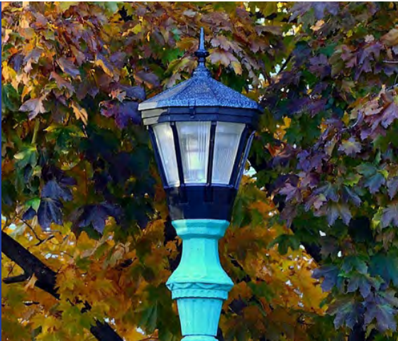
Light fixtures are typically the lantern-style shown here with high hand holes to prevent wire theft.
