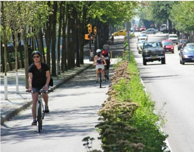
**Figure 18: Maximum Separation Example**
