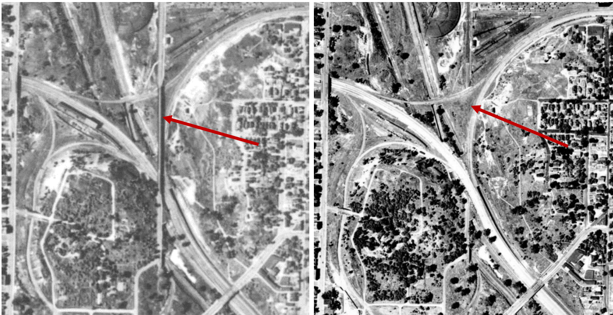
Figures 15 and 16. Aerial images of Westminster Junction in 1940 (left) and 1945 (right) showing the removal of the Westminster Street Viaduct (indicated by the red arrow). 9 (This image was not part of the 1997 evaluation.)
