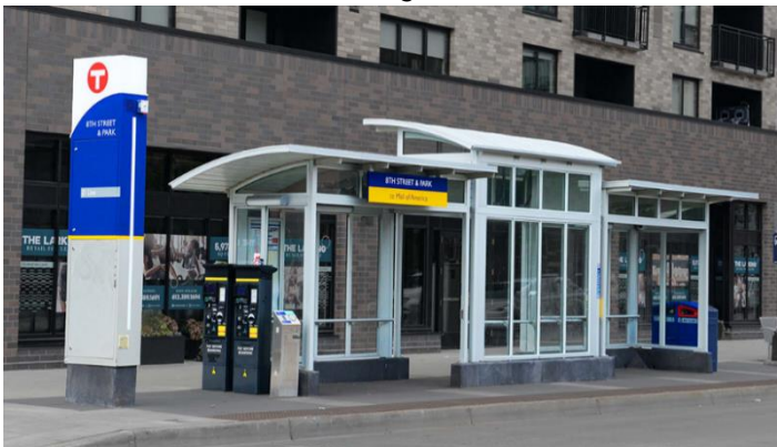
Medium shelter 24 feet long, 5 feet wide, and 9-12 feet high.
