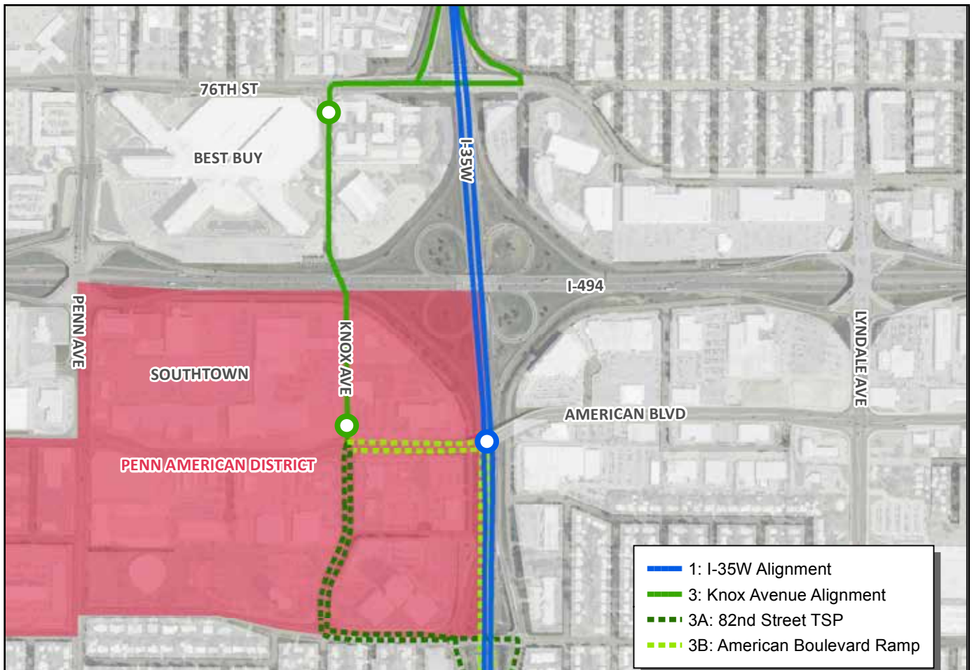
Figure 1. American Boulevard Station Location and Alignment Alternatives
