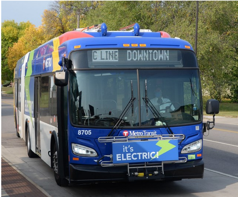
Figure 14 Metro Transit C Line 60-foot articulated BEB
